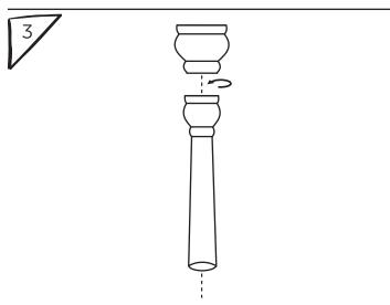
3) Place Part **C** & **D** on Part B & Fix by rotating it counter clockwise.
